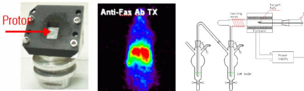
**Figure 1** (Left) Schematic diagram of a  $^{40}\text{Tl}$  target. The target inclined  $45^\circ$  with respect to the direction of the incident beam. Cooling water flows both front and back faces of the target. (Middle) Anti-Fas mediated hepatic apoptosis image using Annexin V labelled with  $^{124}\text{I}$ . (Right) Schematic diagram of  $^{124}\text{I}$  a dry extraction system. Figure available in colour online at [www.interscience.wiley.com](http://www.interscience.wiley.com)
